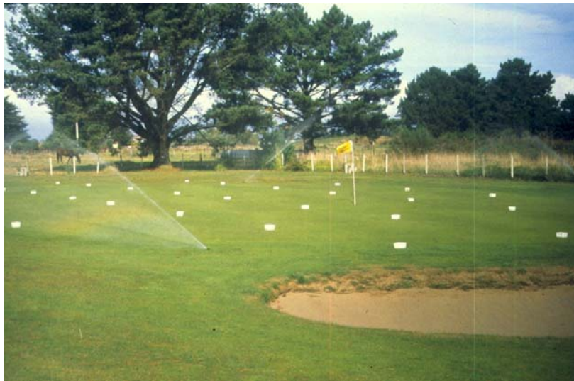
Fig 2. Using catch cans to check the uniformity of watering
