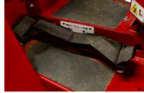
FOOT PEDAL CONTROL A more traditional style foot control for forward and reverse functions.
