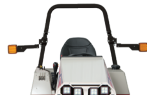
DIRECTIONAL HAZARDS Directional LED signals/blinking hazards.
