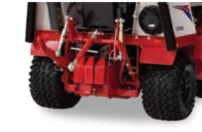
3-POINT Add non-PTO powered implements to the rear with the Category One 3-Point Hitch.
