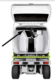
Easy rear access to the hydraulic components such as the service pump, drainage points and **the grass grid can be removed for cleaning.**
