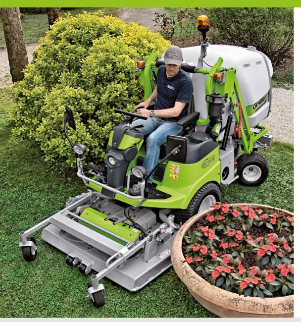
**FD 13.09** is a compact mower with a very narrow wheelbase, **equipped with power steering and a turning radius of only 31 cm.**
