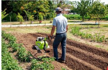
Grillo rotavators are used for tilling even very hard and stony soil to a considerable depth. The user can adjust the tilling depth by putting more or less pressure on the spur and adjusting its height.
