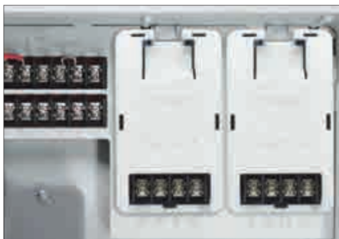
12-station configuration with two 4-station modules (EMOD-4)
