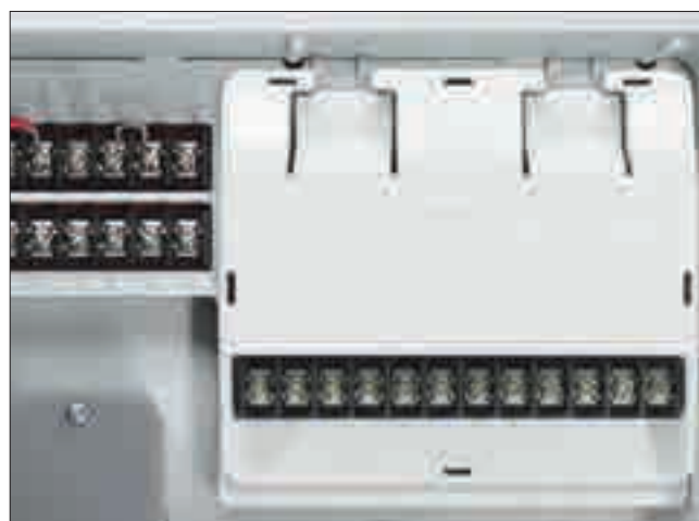
16-station configuration with one 12-station module (EMOD-12)
