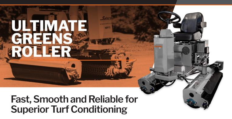
The HP11 Roller is built for fast, smooth, reliable turf conditioning with dual drive oscillating roll and articulating steering. It delivers firmer fairways, faster green, smoother ball rolls. With a high-performance hydraulic pump, the HP11 reaches 11.9 MPH, maintaining consistent pressure.
