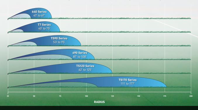
**DID YOU KNOW?** With a radius capability of 177 feet, one TS170 Series sprinkler is capable of covering the entire width of a traditional football field. Only six TS170 sprinklers are needed to cool and wash down an entire field.
